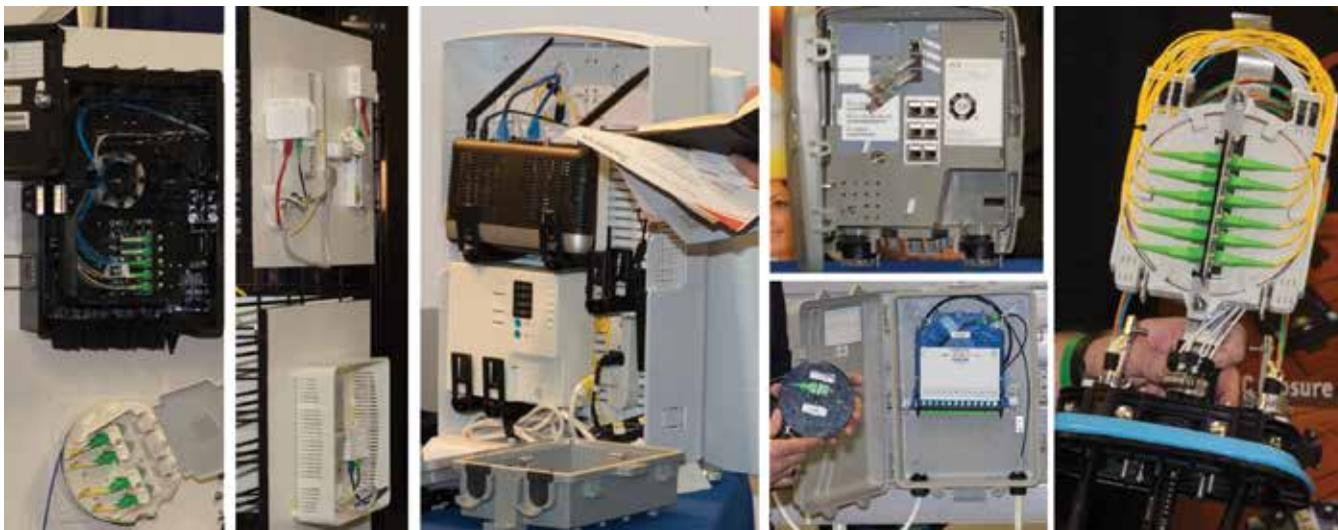
Boxes for handling fiber in tight places come in almost any shape and size imaginable. Shown (left to right) are enclosures from Opterna, iPhotonix, Primex, Zhone (top), Clearfield (bottom) and Preformed Line Products.
