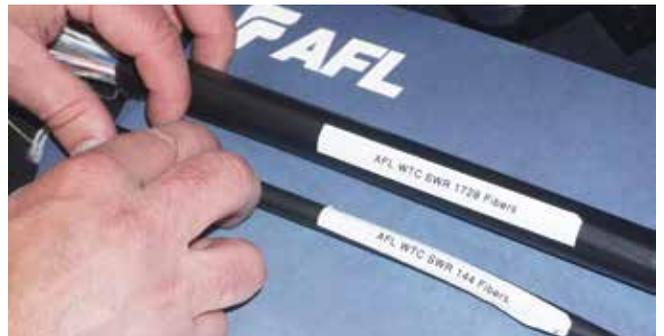
AFL's new 1,726-fiber cable is remarkably thin but quite a handful to work with. One innovation to make life easier for technicians: The fiber bundles can be parsed in the field like spiderwebs.
