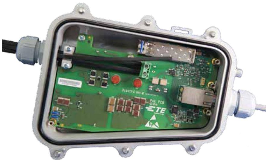
Figure 2: A PoE Extender converts GPON signals to PoE and can extend PoE up to 3,000 meters.
