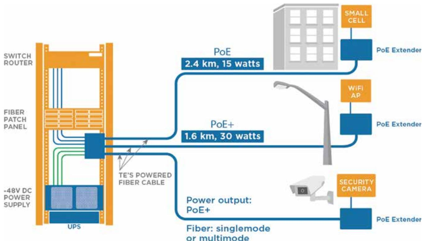
Figure 1: A powered fiber cable system
