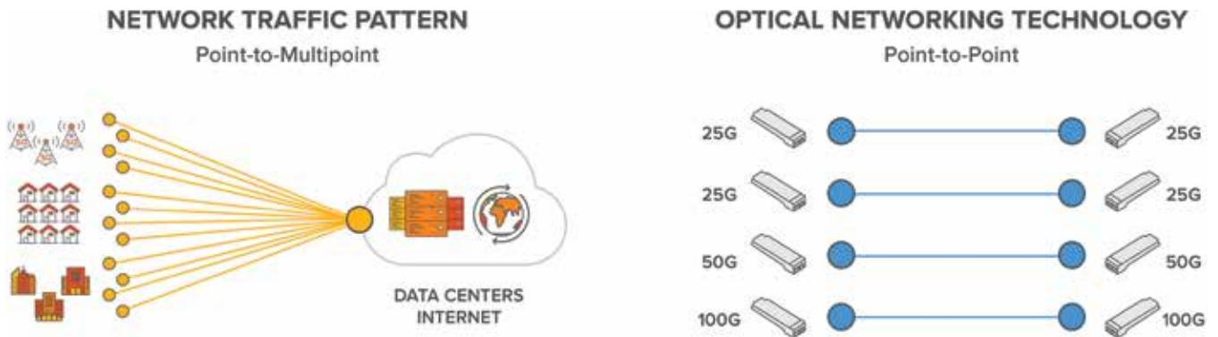
Figure 1: Point-to-point optics vs. hub-and-spoke traffic
