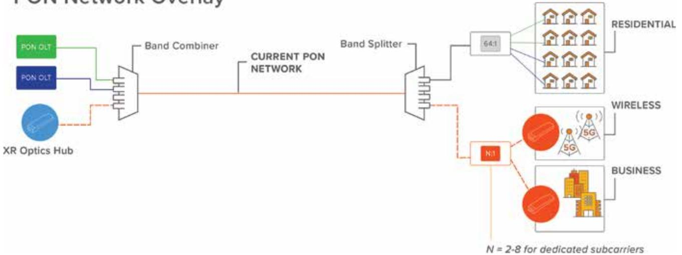
Figure 3: Typical deployment of XR optics over an existing PON infrastructure
