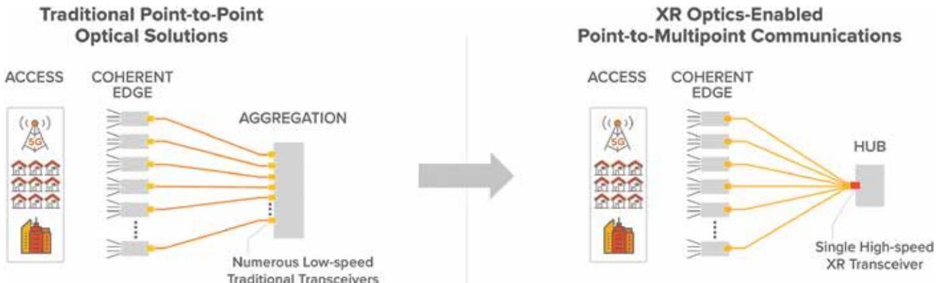
Figure 2: XR optics point-to-multipoint connectivity
