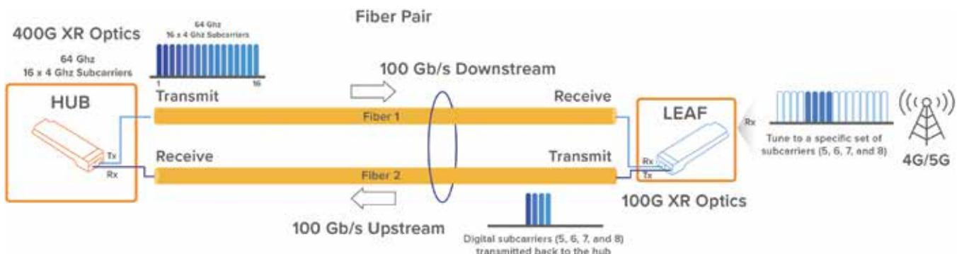
Figure 4: XR optics over a fiber pair
