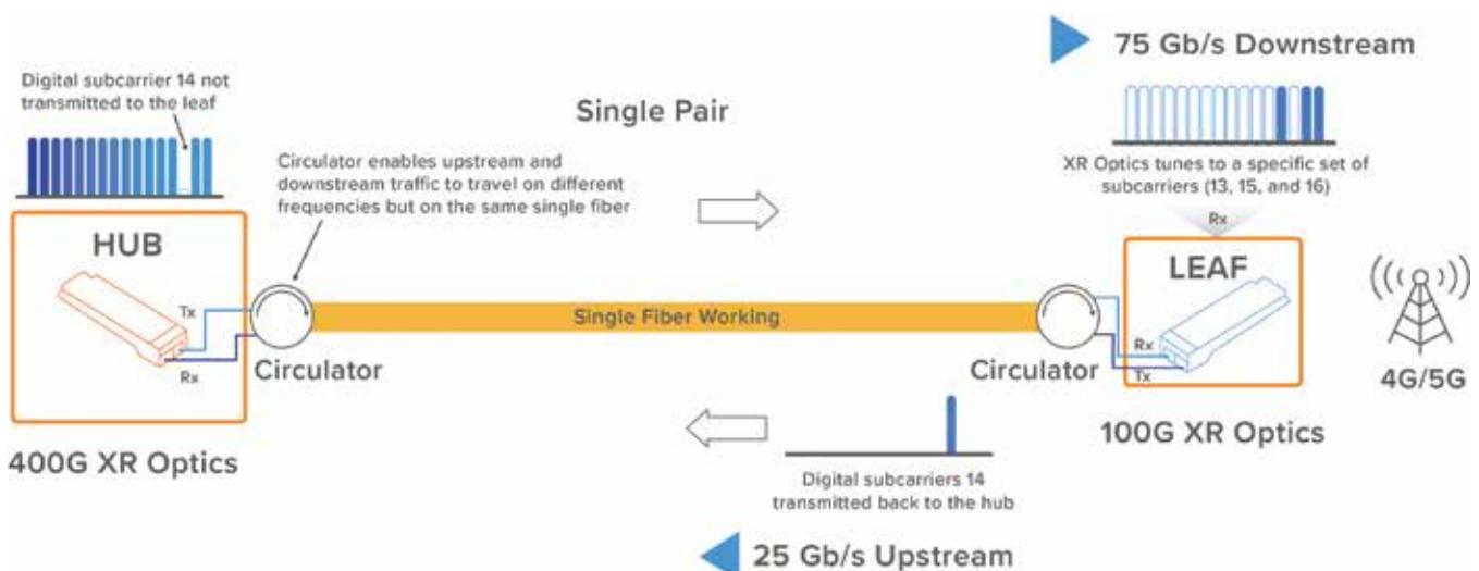
Figure 5: XR optics over single fiber
