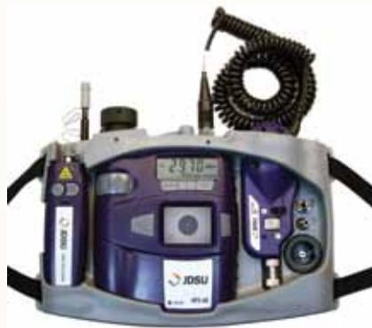
An integrated OPM/inspection device..
