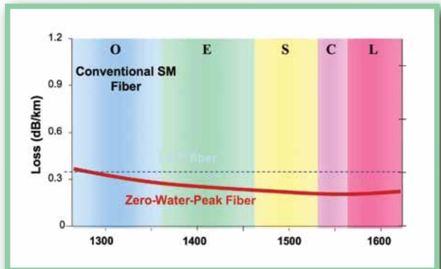
Chart 3: Zero-water-peak fiber has no additional loss in the E-band.
