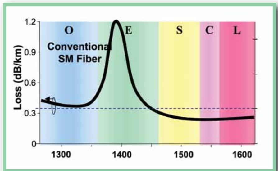
Chart 1: Water-peak loss in a single-mode fiber
