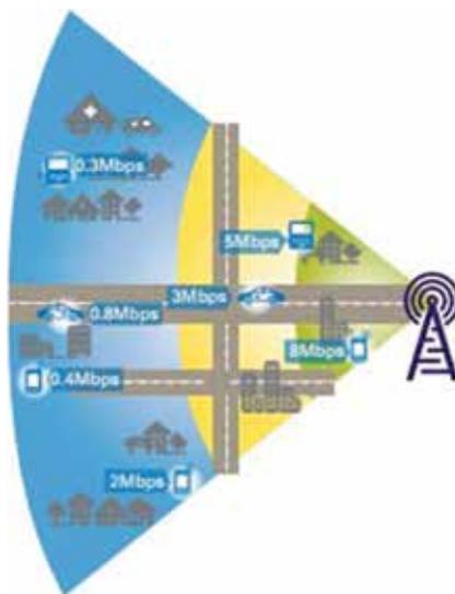
Figure 2: Snapshot of instantaneous user throughput within a typical 10 MHz sector
