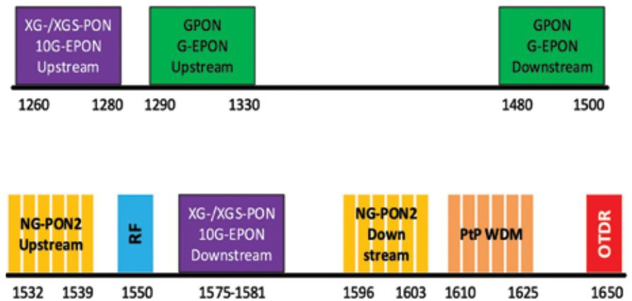
Figure 1. Next-generation PON wavelength allocations
