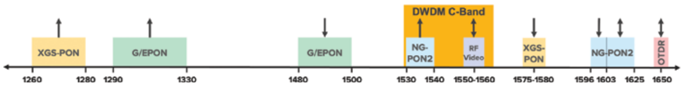
Figure 4. PON and C-Band DWDM operating spectra.
