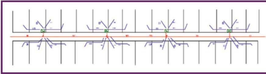
Figure 5: Spliced-feed design: Each terminal is spliced at its placement point.
