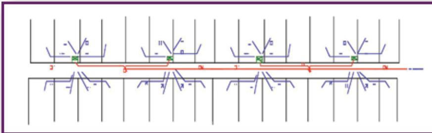
Figure 6: Double spliced-feed design: Two splice points are placed inside the study area.
