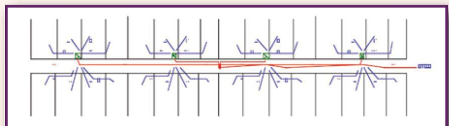
Figure 4: Direct-feed quad design: All terminals are spliced in the center of the study area.
