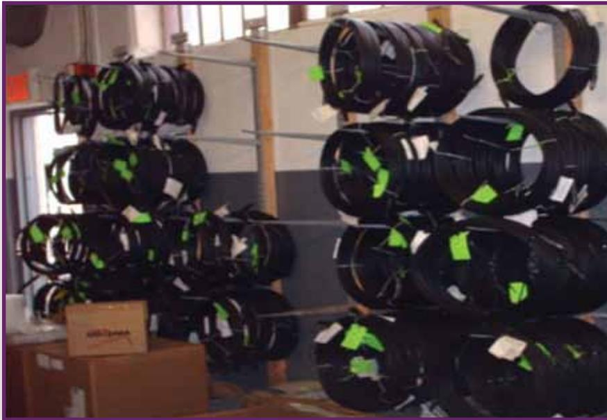
A connectorized OSP solution requires keeping drop cables in many lengths available at all times.
