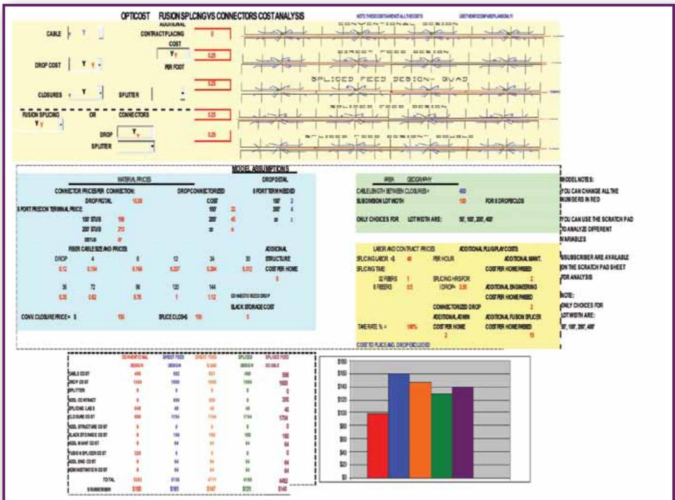
Figure 7: Cost model for evaluating splicing-versus-connectorization decisions in the outside plant
