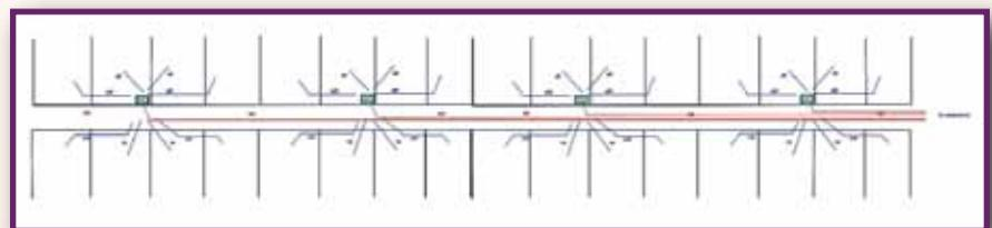
Figure 3: With the direct-feed design, all terminals are spliced where the cable enters the area.
