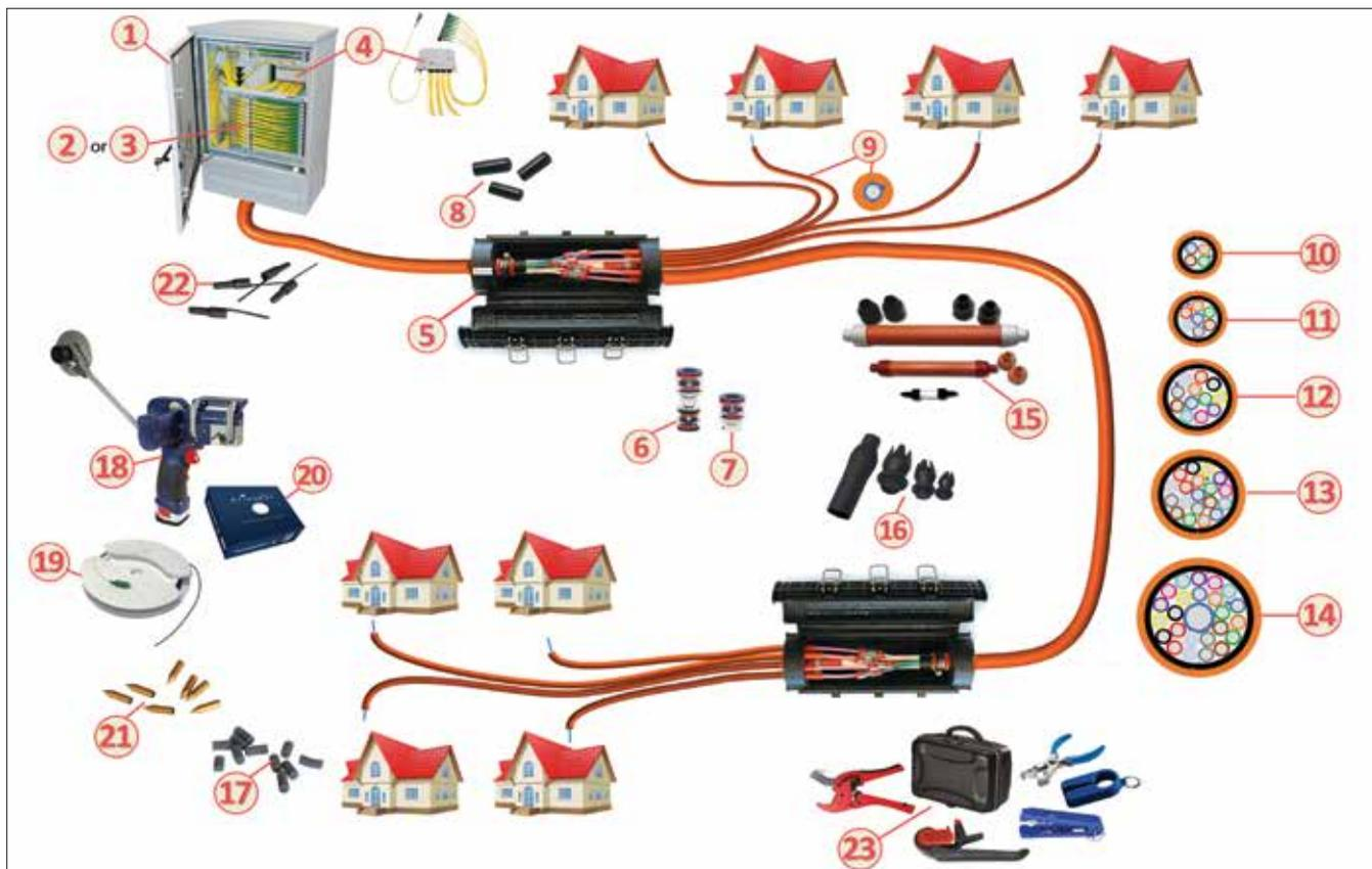
Figure 2: Typical blown fiber system schematic for FTTH
