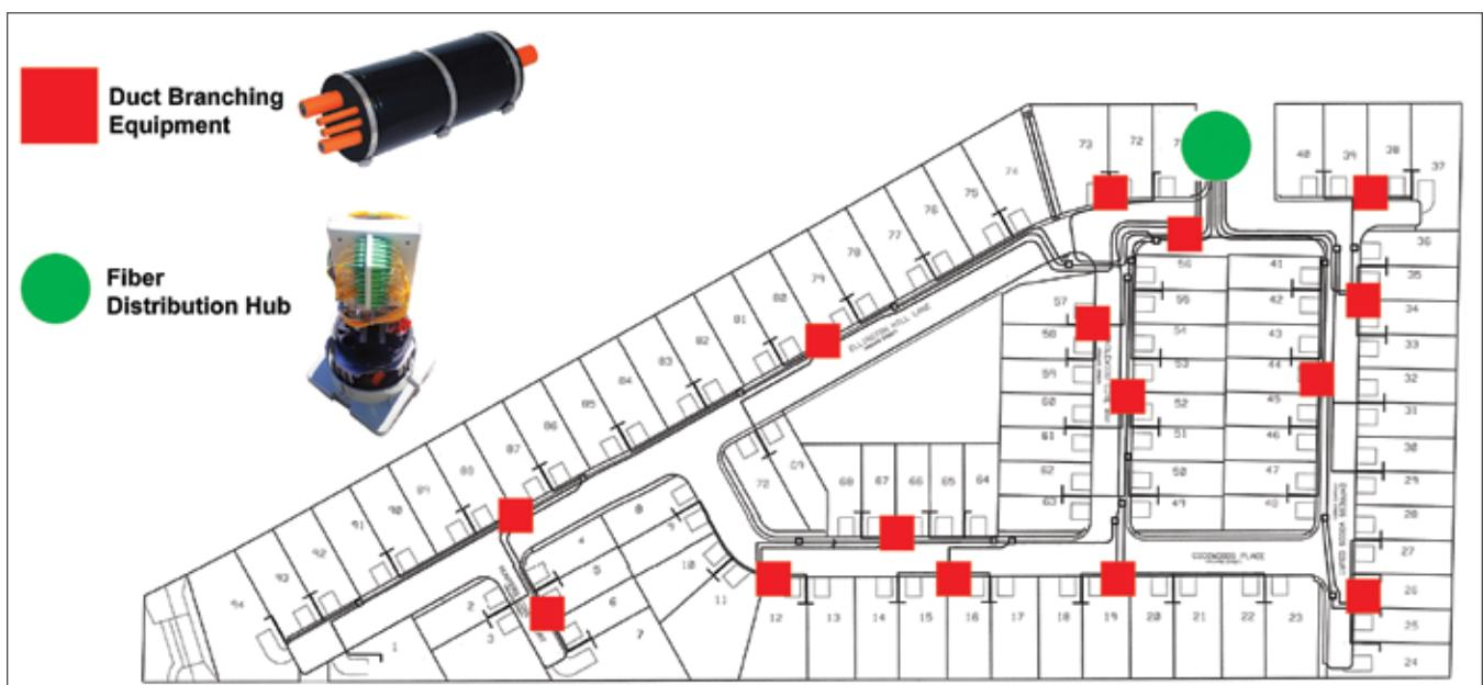
Figure 5: Fiber optic broadband connection of Single Family Units (SFU) in a residential area
