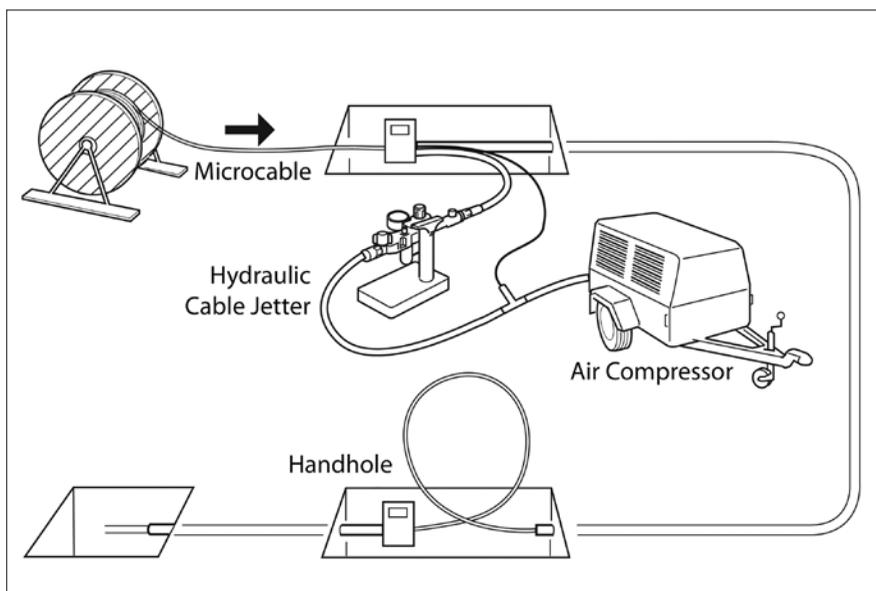
Figure 1: Schematic of blown microcable system components
