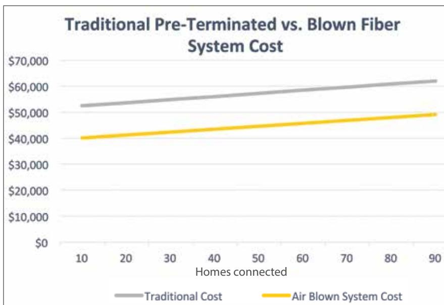
Chart 1. Traditional system cost versus cost of Hexatronic blown fiber system
