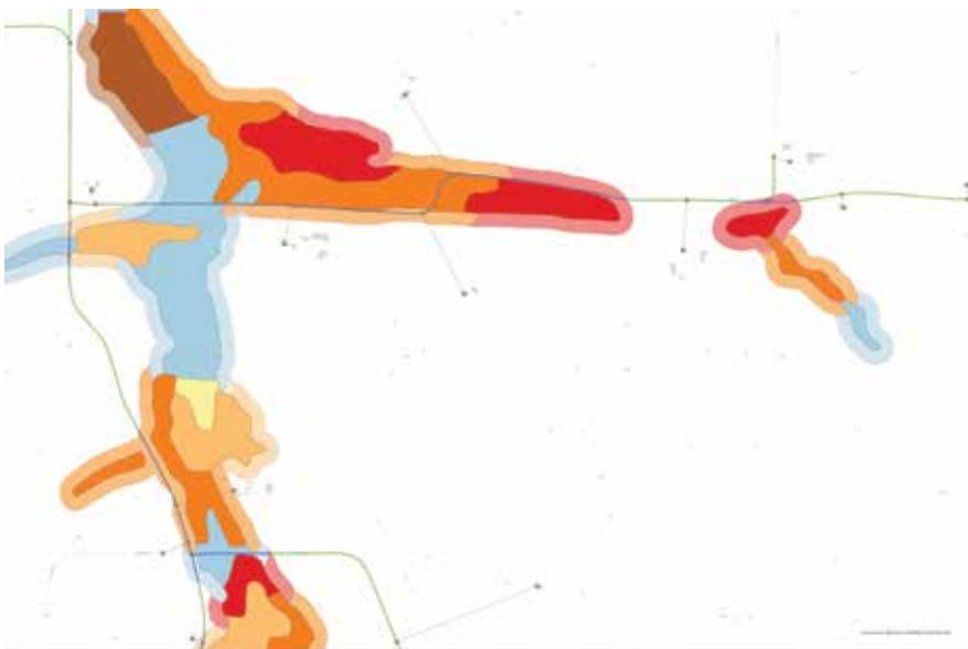
In rural buried fiber construction, wetlands are often bored to reduce environmental impact. Boring can cost three to four times more than plowing. Wetlands can have a significant impact on the accuracy of probable cost to build an area.
