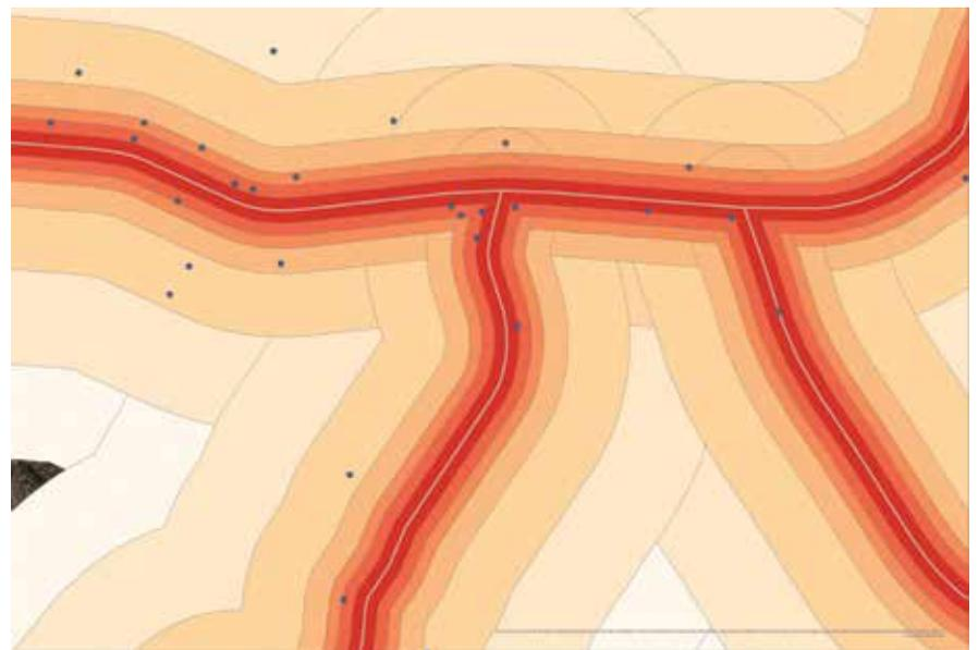
The cost to place a drop can be one of the most expensive costs per foot, per establishment. By overlaying the roads and address points with incremental buffer zones representing the distance from the road centerline, software can be used to estimate the drop footages quickly and with greater accuracy.
