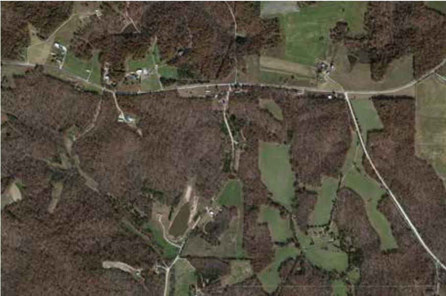
Aerial photography of a proposed serving area shows larger features that can impact the cost to build, such as rivers and canyons. However, finding and tabulating wetlands that may have a larger impact on the overall cost to build is time consuming. Tools within GIS can save time to obtain the necessary information and provide greater accuracy when planning broadband network expansion costs.
