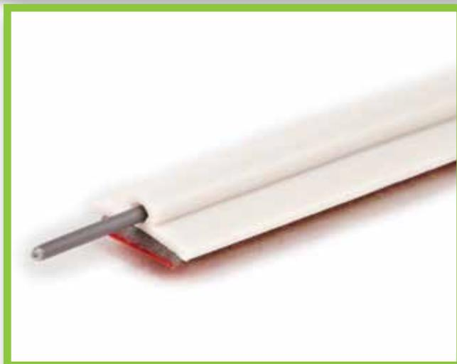
The One Pass Mini Fiber Pathway connects to a hallway distribution cable and is routed inside a living unit to a wall outlet positioned near an ONT. The One Pass Mini uses exclusive 3M adhesive technology that ensures reliable installation on a wide variety of surfaces, even painted or sealed concrete where stapling cables isn't an option.
