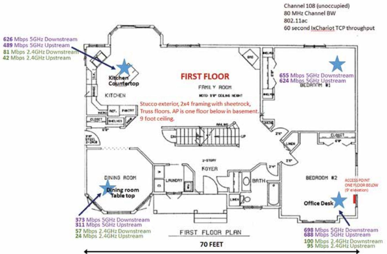
Anticipated wireless coverage in a typical house equipped with a Calix GigaCenter gateway
