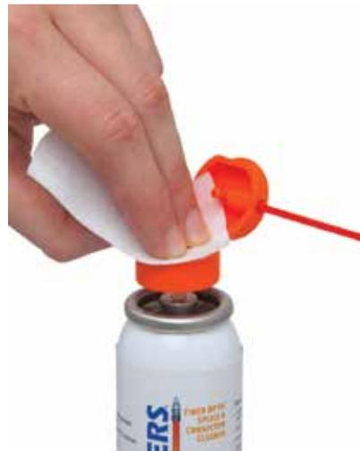
Alcohol is no longer suitable for cleaning modern fiber optic networks. A much better choice that will lower network maintenance costs is a nonflammable, water-free, fast-drying fluid packaged in a sealed, nonrefillable container. Here, a lint-free fabric wipe is dampened from a convenient pump bottle dispenser.
