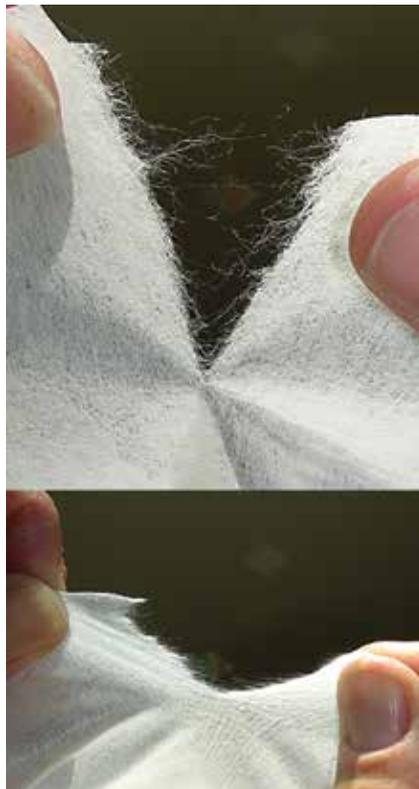
Many field techs are provided cheap paper wipes to clean their end faces, but these can cause static and leave particulate on the end faces. A cheap paper wipe (top) is easily ripped, and many fibers are released, but a stronger, cleaner fabric wipe is much stronger, resists shredding and is less likely to leave fibers on the end faces.
