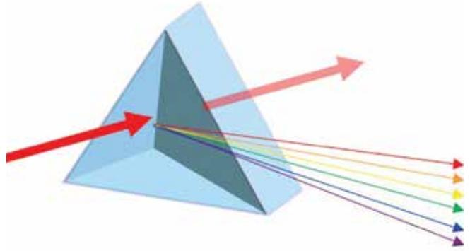
Translucent liquid contamination is particularly troubling for fiber networks because the fluid changes the refractive index of the fiber, which can spray different optical frequencies unpredictably.
