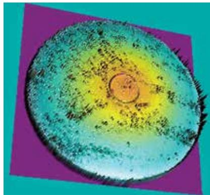
Most field techs carry optical inspection scopes to examine end faces, but interferometers offer a richer, more detailed look at the contamination in all three dimensions.
