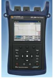
laser source and visual fault locator.
