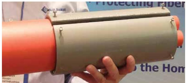
Many vendors showed polymer conduit – typically high-density polyethylene (HDPE) – and MaxCell showed fabric ducts with real-world, mixed-technology deployment examples. These pictures show Blue Diamond Industries conduit for fiber optic cable networks that need ducts-within-ducts (1/2 inch to 6 inches in diameter) and extra armoring. Options include prelubrication, preinstalled pull tape, preinstalled cable-in-conduit and a toneable wire.
