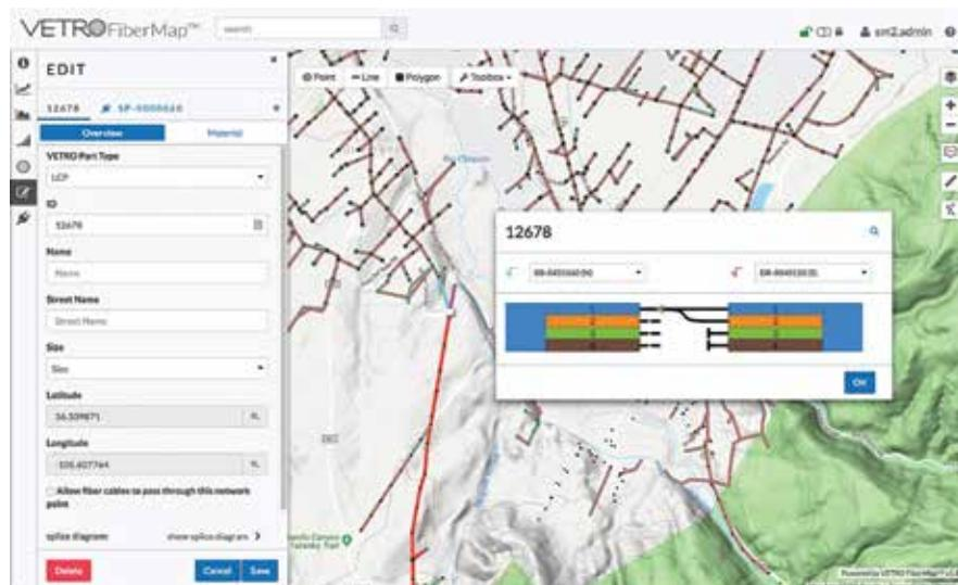
Sample splicing diagram in VETRO FiberMap
